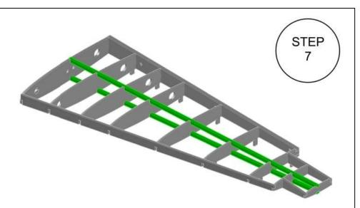
Place first top spar over rib notches. Check perfect fit and glue in place with medium CA.
