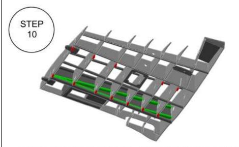
Create main spar pocket by gluing 1/2"x1/4" balsa sticks between ribs, by sliding the main spar protected to avoid get glue to W17. Check plans for detail.
